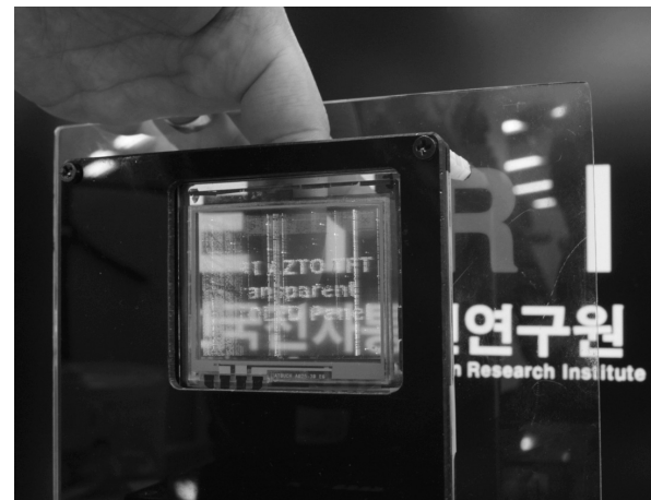
Fig. 14 AMOLED panel using the top gate AZTO TFT back-plane.
